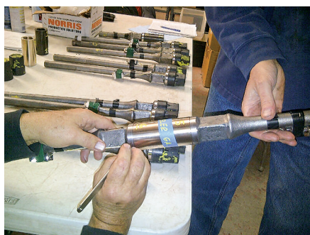
Fig. 2. New prototype couplings and a controlled makeup/breakout test setup.
