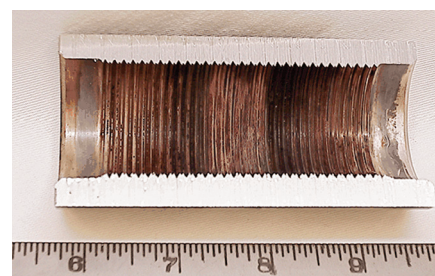
Fig. 6. A cross-section of recovered ToughMet coupling.
