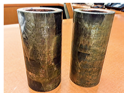
Fig. 6. A cross-section of recovered ToughMet coupling.
