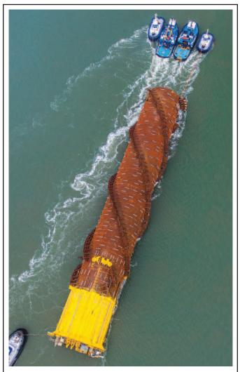
The 584-foot long hull is shown here in February 2014 as it was making its way through Aransas Pass along a 515-nautical-mile journey from Gulf Marine Fabricators' facility in Ingleside, Tx., to Mississippi Canyon 724. Once on location, the hull was upended, ballasted and moored in position.
